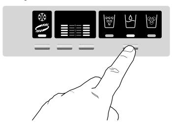
To reset the display, press and hold drinks dispenser button for 5 seconds. The warning will deactivate and the display light will return to blue.
